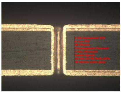
3 mil mechanical Drill, 8 mil core FR4, No Plasma, Permanganate Desmear, 3 min microetch, Double Cuposit, 10 min via fill flash plate, 45 minute pulse plate
